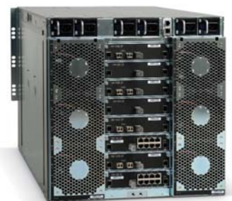
Figure 2: Back view showing 6 x 10 Gbps, 16 x 1 Gbps uplinks, and 16 x mini SAS connectors 4 x 6 Gbps to external fabric storage devices.
