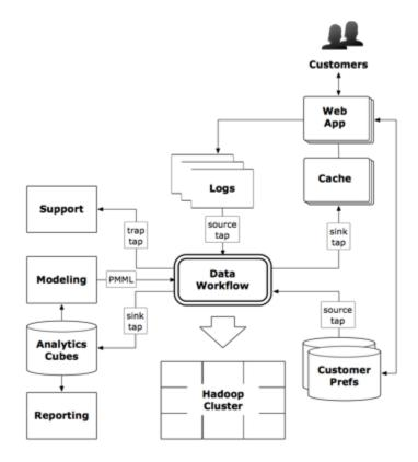
By using Cascading Pattern, predictive modeling can now be exported as PMML from a variety of analytics frameworks, then run on Apache Hadoop at scale. This saves licensing costs while allowing for applications to scale-out and allows for predictive modeling to be integrated directly within other business logic expressed as Cascading apps.
