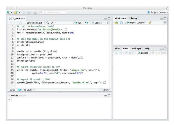
This will execute the R script and create the predictive model. The last line saves the predictive model into a file called "sample.rf.xml" as PMML. If you take a look at that PMML, it's XML and not optimal for humans to read, but efficient for machines to parse:
