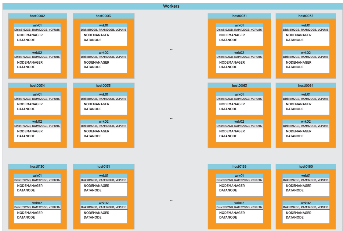
Figure 4: The Worker virtual machines (wrk01-02) and their resident Hadoop processes with two virtual machines per host server.
